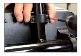
**Step 8:** Pull motor wires through frame. Remove E-Box and set aside.
