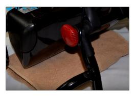
**Step 10:** Push motor wires through frame. Left motor goes to white marker & right motor goes to black marker.
