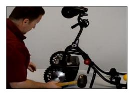
**Step 18:** Install motor sleeve screw (one for each motor).
