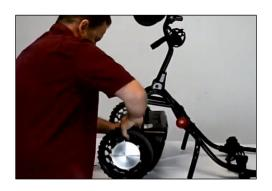
**Step 5:** Disconnect the motor wires by pulling them apart.
