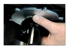
**Step 3:** Remove the screw that secures the motor to the frame using the #2 Phillips screwdriver.
