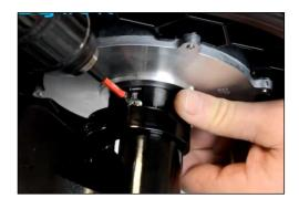
**Step 4:** Using the rubber mallet, tap the motor/wheel assembly outward towards you. Remove both left & right motors.
