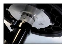
**Step 17:** Using the rubber mallet, tap motor inward.
