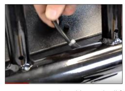
**Step 11:** Note: The rubber seal will fit over hole and frame.
