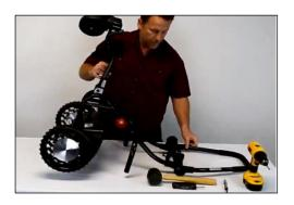
**Step 1:** Loosen the motor sleeve clamp using the 4 mm Allen hex wrench.
