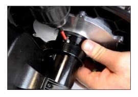
**Step 19:** Slide down motor sleeve clamp and tighten.
