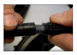
**Step 15:** Put a strip of black (electrical) tape around wires to keep from vibrating loose.
