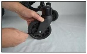
**Step 4:** Install the replacement caster wheel with the 5 mm hex bolt and nut.
