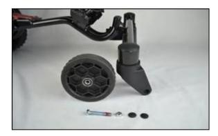
**Step 5:** Adjust the torque for normal rotation. The wheel should achieve roughly 5 rotations on a single spin. Replace caster wheel caps.
