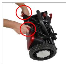
4. As you lift the pull bar up, the front caster wheels will move forward and unit will unfold.
