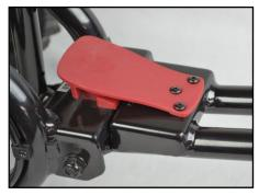
**5th Wheel Check**Check the torque on the hex and Phillips screws
