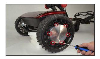
**Step 3:** Pull the wheel off of the motor.
