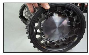
**Step 5:** Rotate wheel clockwise and align the 6 screw holes with the holes on the wheel.
